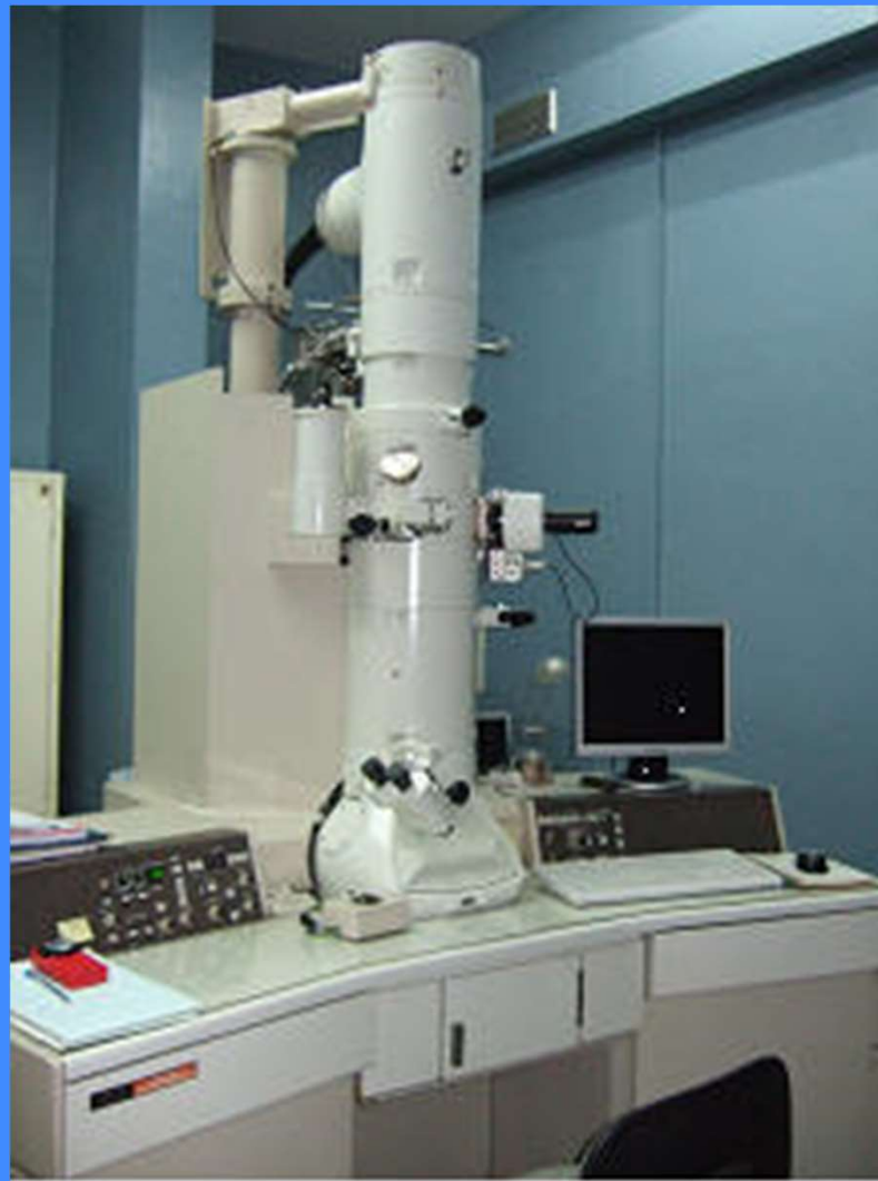
HRTEM JEOL 2011 Resolution: 0.194 nm 200 KeV
