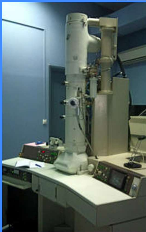
HRTEM JEOL 2000FX Resolution: 0.28 nm 200 KeV
